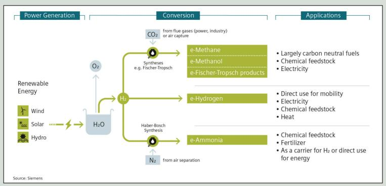
Three pathways of power-to-x: electricity-based molecular hydrogen, ethanol and hydrocarbons, as well as ammonia
